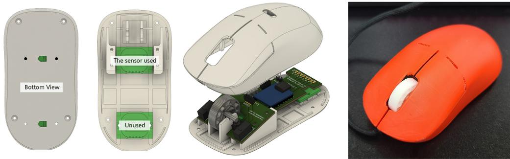
Figure 7: The custom-built mouse hardware design: Only the signal from front sensor was used in this study.
